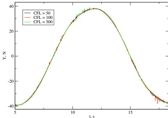
Figure 6: KCS sway force comparison for different maximum  $CFL$  numbers.
