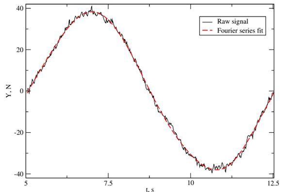
Figure 1: DTMB 5415 sway force signals: raw and Fourier series representation in one PMM period.
