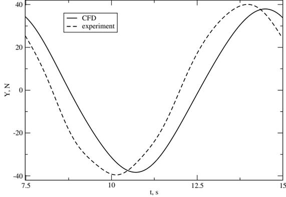
Figure 2: DTMB 5415 sway force comparison.
