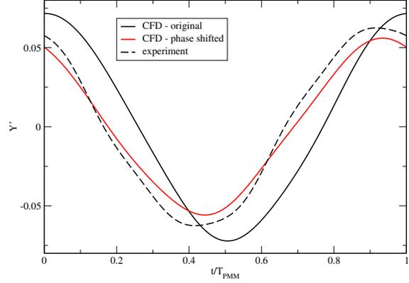
Figure 4: DTMB 5415 dimensionless sway force.
