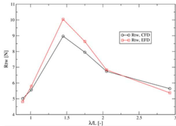
**Fig. 4** Mean total resistance in waves comparison
