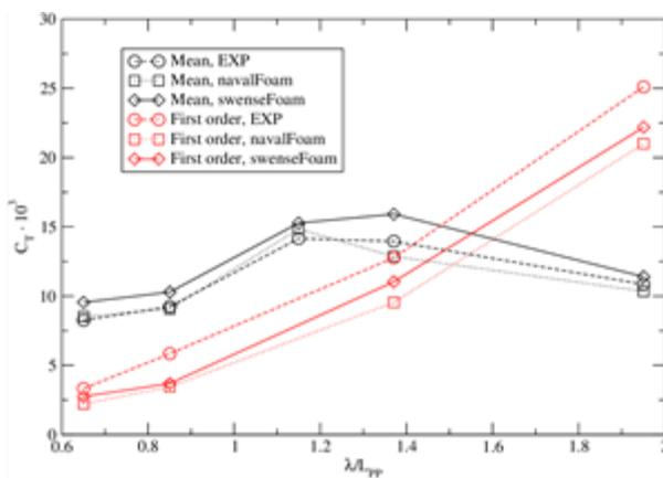
Fig. 7 Resistance coefficient RAO, head waves KCS
