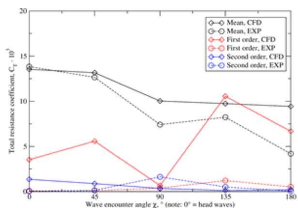
Fig. 12 Resistance coefficient RAO, oblique waves KCS
