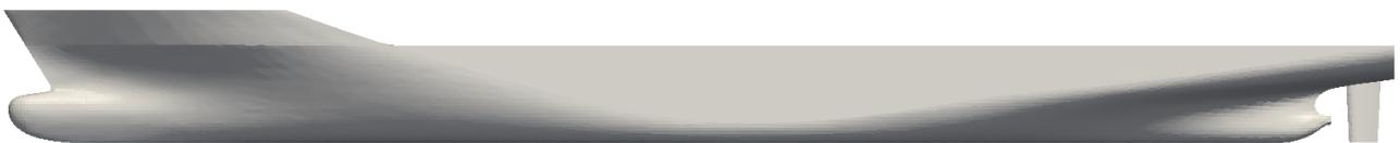
**Fig 3.** KCS hull with rudder, side view.
