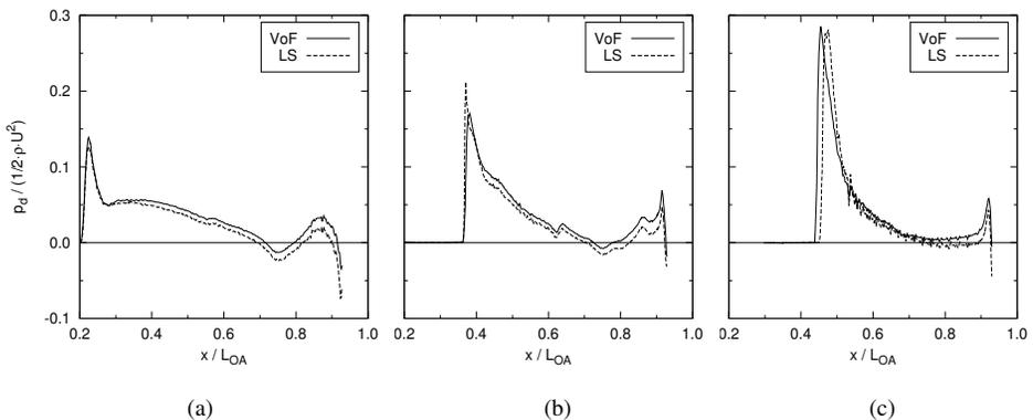
**Figure 5.** Non-dimensional dynamic pressure along three longitudinal cuts (10% (a), 50% (b) and 80% (c) of the hull half-width) on the hull surface at the highest design speed. Solid line: VoF; dashed line: LS.
