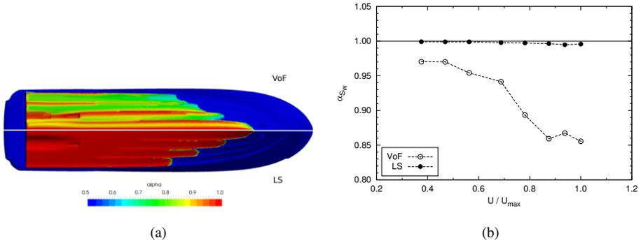
**Figure 4.** (a) Bottom view of the volume fraction on the wetted hull surface using VoF (upper) and LS (lower) at the highest design speed. (b) Volume fraction on the wetted hull surface, both with VoF (o) and LS (●), as function of hull speed.
