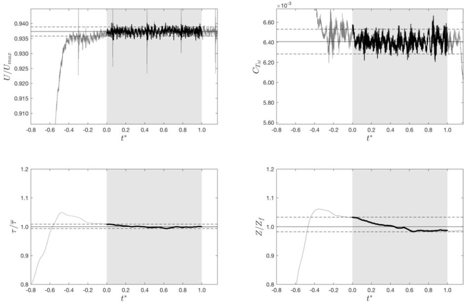
**Figure 2.** Sample time series of adimensional carriage speed (top-left), total resistance (top-right), trim (bottom left) and sinkage (bottom-right). Shaded interval: analysis window; solid black line: mean value; dashed black lines: confidence limits.
