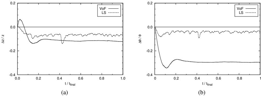
**Figure 7.** Time series of the non-dimensional sinkage (a) and trim (b) during the simulation at the highest design speed. Solid line: VoF; dashed line: LS.
