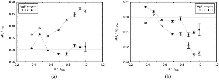
**Figure 6.** Non-dimensional error in the vertical force (a) and in the pitching moment (b) with respect to the towing point. VoF (○) and LS (●) simulations.
