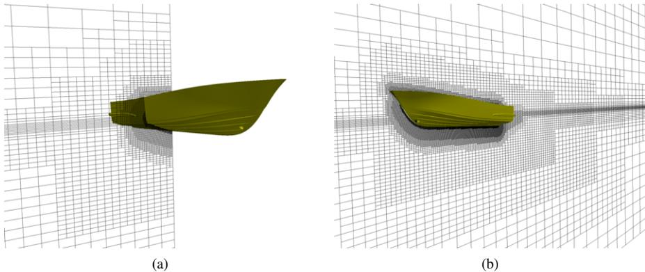
**Figure 3.** Sample grid obtained with the home-developed automatic mesh generation procedure.
