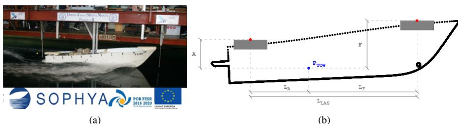
Figure 1. Experimental set up for the calm water resistance tests.
