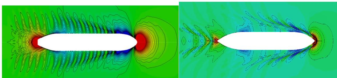
**Figure 3. Wave field of the vessel sailing at 10 knots in load condition 8 (left) and in 14 knots in load condition 3 (right).**
