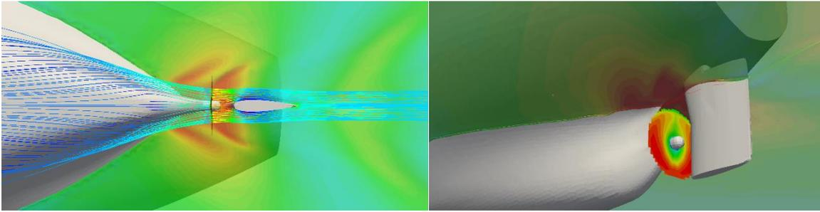
**Figure 4. Streamlines showing the flow through the propeller and around the rudder (left), velocity magnitude on the propeller plane (right).**
