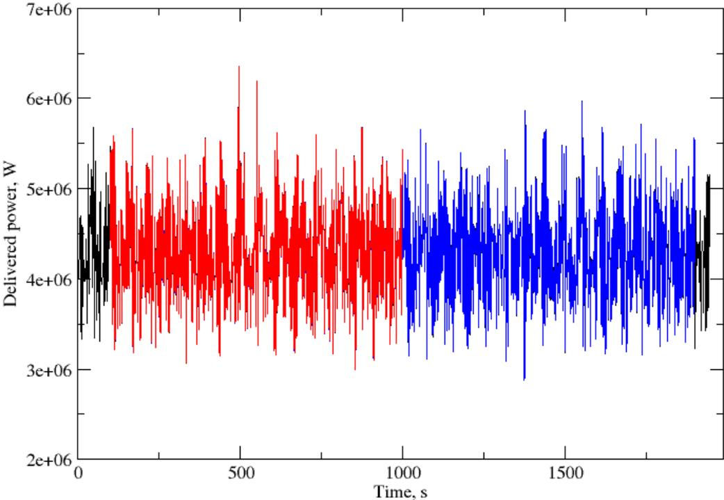
**Figure 8. Time signal of the power delivered to the propeller during a simulation in irregular waves for load condition 3, trim 2.0 metres. The black line is the entire simulated signal, the red is the signal from 100 to 1000 seconds, and the blue from 100 to 1900 seconds.**
