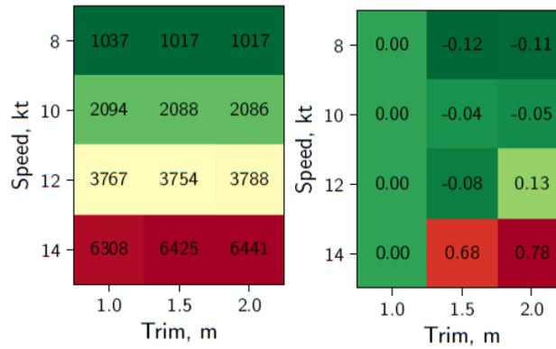
Figure 6. Power in kW (left) and fuel savings in tons per day with respect to trim of 1.0 m (right) for different speeds and trims for Load condition 3.
