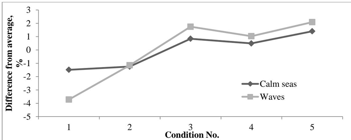
**Figure 10. Comparison of power trends in percentages of the average value between calm seas and irregular waves results for speed of 12 knots.**
