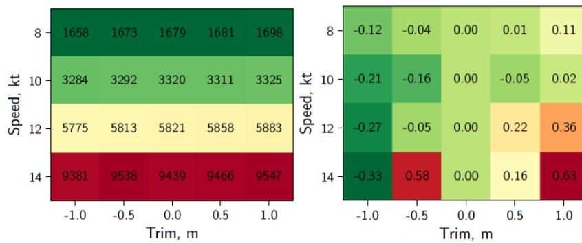
Figure 7. Power in kW (left) and fuel savings in tons per day with respect to even keel (right) for different speeds and trims for Load condition 5.
