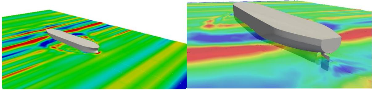
**Figure 9. Simulation of a vessel sailing in irregular head waves.**
